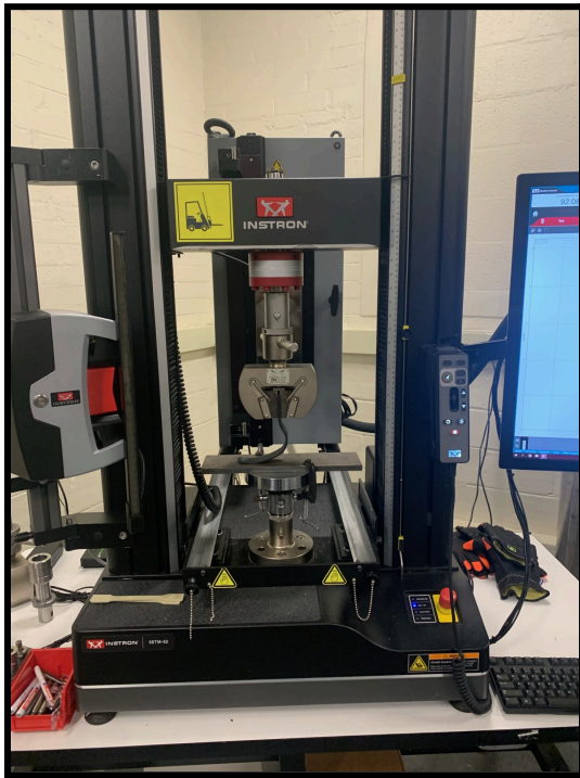
Picture of the PLA running blade in the Instron Compression tester
