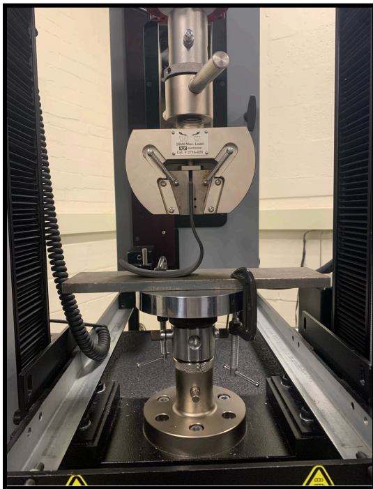
Picture of Onyx running blade after some Compressive load has been applied
