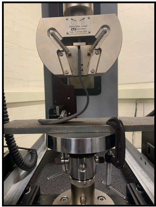
Picture of the Onyx running blade before force has been applied
